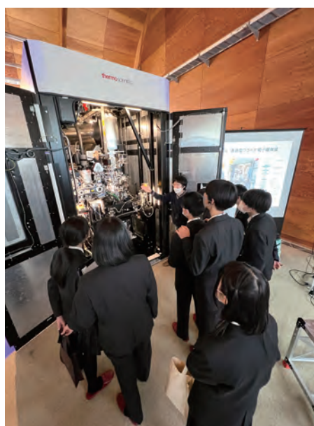
▲ The three cryo-electron microscopes (cryo-EMs) housed in the Central NMR Complex, aligned in a row. On the far right with its enclosure doors open is the latest, state-of-the-art cryo-EM that is equipped with an electron emission gun with an acceleration voltage of up to 300kV. To its left is the sample preparation area and computers for analyzing the data. The two boxed areas on the far left each houses a 200kV cryo-EM.
